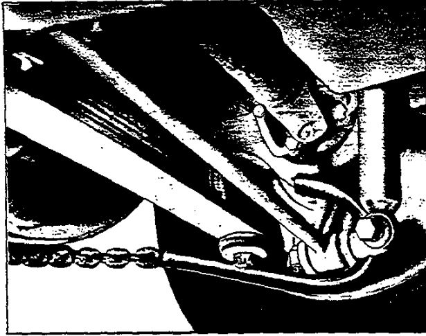
Fig. 3—Connect Hooks Outboard of Shock Bracket
