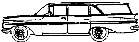
Model 17-1835 Nomad — 4-door, 6-passenger, 8 window Station Wagon, drop gate in rear with retractable window.
