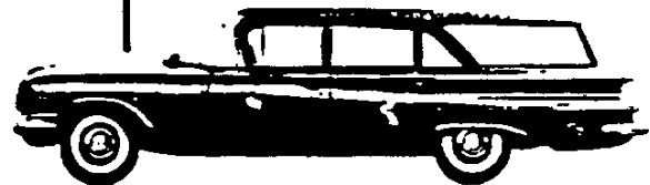
Model 11-1235 Brookwood — 4-door, 6 passenger, 8 window Station Wagon, drop gate in rear with retractable window.
