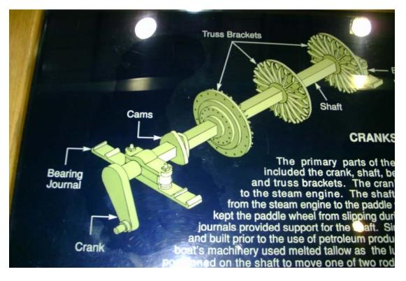
The truss brackets (diagram above) held the spindles for the paddle wheel. Lubrication for this assembly pre-dated petroleum products so lube was provided with animal tallow.
