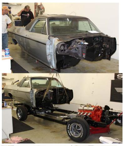
Always a big milestone when the reworked body meets up with the fresh frame and running gear.
