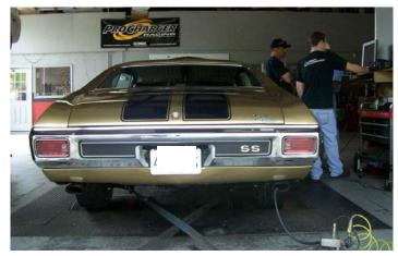
Above: Danny's '67 was first out of the gate with an impressive 370 hp at the rear wheels and 490 ft lbs of torque.
