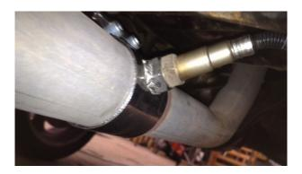
that ordeal includes a trip to the muffler shop to have the fitting welded in. Hassle. Although I do have a welder, and welded my last bung in, I thought I would try the easy route to see how it worked. The kit that I used included a nice band clamp, gaskets, and hardware for installation. Simply drill a hole in the spot you would like it, apply the gasket, and clamp it on. Worked very well, and leak free-Easy!
