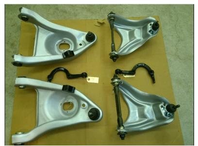
The Front Conversion Brake line kit includes the left & right brake lines and the 2 small lines that go from the Master Cylinder to the Combination Valve (these 2 lines came in the front conversion kit too). I ordered new clips also. Shown are the clips for the front lines and the front to rear line. I repainted the upper and lower control arms after the new ball joints and bushings were installed.
