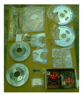
Here are the parts included with the rear conversion kit. Backing plates, Caliper mounting bracket, bolts, and Caliper adjustment shims, Calipers, Braided Caliper hoses and hardware, 11" Discs, E-Brake cables. The T-Block and mounting bracket were purchased separately. The axle brake lines and flex hose were part of the brake line conversion kit.
