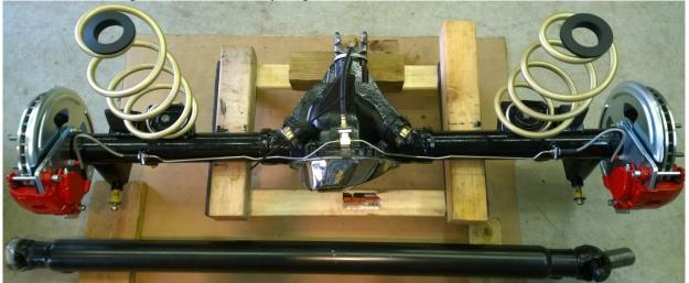
After installing the cover and adding 2 quarts of gear oil we just rolled the completed project under the car, put two floor jacks under the shock mounting brackets and a bottle jack under the center and lifted it right in place. After greasing up the polyurethane bushings and thrust washers we installed the upper and lower control arms. You are going to have to use all 3 jacks for positioning and a little muscle to get everything lined up, definitely a 2 man job.
