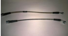
I knew what I needed to solve this dilemma and after a few hours of researching the internet I found the hoses I needed. A hose with a 10 millimeter 45 degree angle banjo fitting on the caliper end and a 3/8-24 inch thread female fitting on the other
