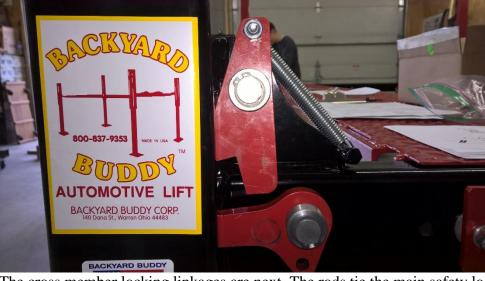
The cross member locking linkages are next. The rods tie the main safety lock dogs together so all 4 will lock into the leg slots at the same time as the lift raised and unlock at the same time when you are ready to lower it.
