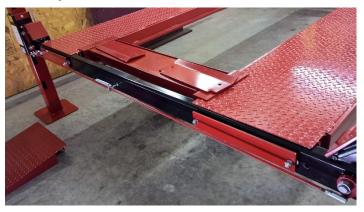
The assembly looks like this and will be on each end of the cross members. Heim ends on both ends of the threaded rods make adjusting them to the main lock dogs easy and the spring in the middle keeps tension on the main lock dogs so they lock into the leg slots automatically as the lift is raised.
