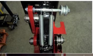
Assemble the 4 secondary lock dog assemblies to each corner of the cross members. The lift cable will ride on the small pulley and engage the lock tab when the cable goes slack. The cables will go slack when the lift is lowered on to the main safety log dogs. It will also engage if for some reason a cable would go slack or break keeping that corner of the lift from falling. Another safety device that I liked about this lift.
