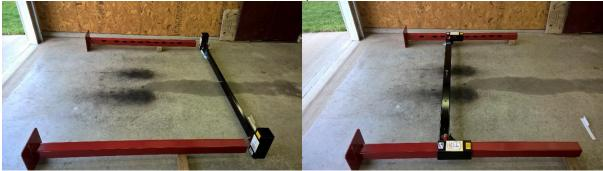
Lay out the leg assemblies on the floor supported by 4 X 4's on one end. The slots in the legs should be toward the top of the leg, the leg with the hydraulic system mount bracket will be in the left front corner. Next slide the cross members onto the leg assemblies locking them into position with the main safety lock dogs on the cross members in the 4<sup>th</sup> slot from the bottom of the leg.
