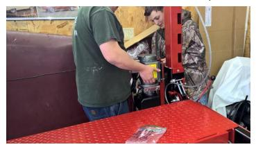
The last item to install before the final adjustments is the hydraulic power unit and hose. The unit comes with a quick disconnect fitting to attach to the hose that goes to the power unit and the other fitting to the hard pipe on the side of the ramp that goes to the hydraulic cylinder underneath.
