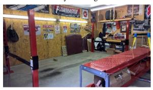
Stand up both assemblies and position them in the place that you want the lift to be. After the ramps are attached they will not be easy to move (unless you purchased the wheels) so they need to be as close as possible to where you want it. Also both front legs and cross member (hydraulic end) will need to be at least 4 feet from the wall (I will explain later).
