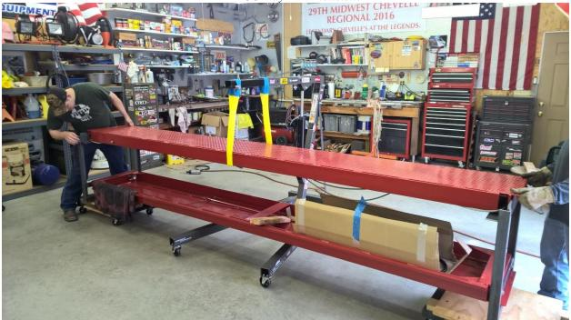
Here's where the engine hoist come in.......Position the hoist in the center of the ramp with the hydraulic cylinder, take the weight off the shipping legs and unbolt it. Roll the bottom ramp out of the way and move the ramp into position onto the leg assemblies. Make sure the hydraulic ram hard pipe is on the outside side of the ramp next to the leg with the hydraulic unit mount. Insert the 4 bolts & tighten. 1 ramp down.
