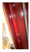
Connect the square rods on both ends of the cross members to the cross members locking assemblies with 2 smaller threaded rods also included with Heim joints. All four main locking dogs are now tied together and will lock together as the lift is raise and unlock together with the main safety lock dog release handle to lower the lift.
