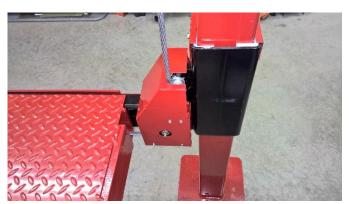
Double check all the safety lock assemblies the cable routing, and that everything is tight and then attach the 4 pulley covers on the cross members. I ran the lift up and down a few times making sure that the main safety lock dogs and the secondary lock dog assemblies were operating correctly before actually lifting the car.
