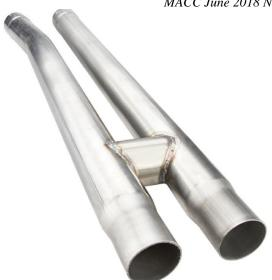
An H-Pipe is also shaped like its namesake and relies on exhaust expansion to balance the cylinder banks. A small section of tubing in between the main pipes provides an area for gases to expand into during exhaust pulses. Only a small amount of exhaust flows from one stream to the other as both sides push back and forth in the center section. H-Pipes feature is low restriction, so gains in performance are noticed from low rpm and give the exhaust a deeper, muscle car-like tone.
