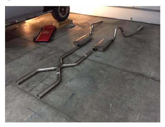
An X-Pipe is, you guessed it, shaped like an x, and allows the exhaust to flow down the path of least resistance. At lower revs, turbulence is formed as exhaust gases try to shuffle past a second column of gases coming from the other side. While always producing more power than
