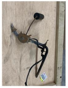
I ordered a new fuel tank, pickup assembly with fuel sender (and a return line provision for the fuel injection), and some foam cushioning material to go between the tank/ body and line the fuel tank straps. I
