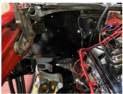
This is a picture of the new steel plate that mounts on the fire wall to cover the holes that are not needed, but also to give support to the fire wall to mount the new air handling unit in the cabin area. You can also see the inner fender well is out and the A/C and heater hose hanging in the engine bay.
