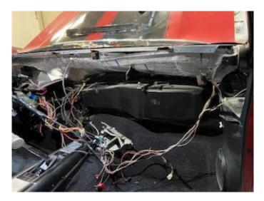
As you can see it looks like a rat's nest after taking out the dash and exposing all the wiring. Next step is taking out the old heater box and controls and removing the blower fan and plenum on the engine side of the firewall. None of this is hard, it's just time consuming.
