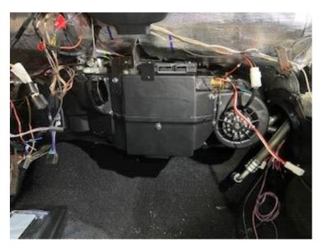
Here is a picture of the new air handling unit that fits under the dash. You also can see the A/C line stub into the cabin area. These lines have to be installed before installing this unit. This was just a test fit to make sure the unit would fit and to make sure all the holes needed were in the right place for mounting.
