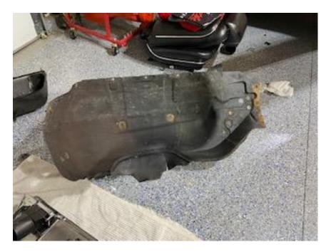
The inner fender well must have been taken out when the car was painted over 25 years ago because it was missing about 5 bolts that held it in place. As you can see, it looks pretty rough. After a visit to the car wash and a can of brake cleaner, it was clean but in dire need of some paint. A coat of POR15 to address the rust and then about 3 coats of spray paint it looks way better and was ready to reinstall when needed. The bolts that were holding it into place on the
