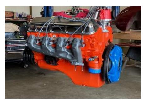
After pulling the old engine out of the car we were able to paint and reuse a lot of exsiting parts. As you can see everything looks brand new and the exhaust manifolds turned out great. I used POR15 high temp spray paint with a high gloss clear spray sealer on the manifolds. After that, the engine was ready to run test on the engine stand. Not to my surpise, it sounded great and I know now I have a engine that will last a very long time.
