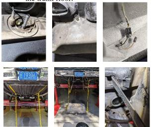
Now that all the tank connections are removed it's just a matter of removing the old tank.
