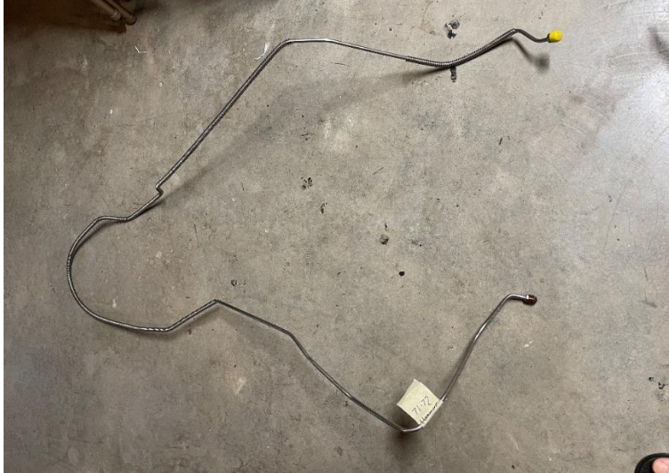
1971-72 Hardtop stainless steel brake line from front combination valve to rear axle. $30
