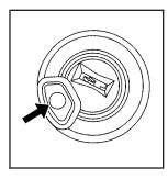
The ignition key cannot be removed from the ignition of manual transmission vehicles unless the key release button is used.
