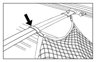
15. Wrap the hook and loop strap around the cross bar as shown to secure the middle portion of the cargo net.
