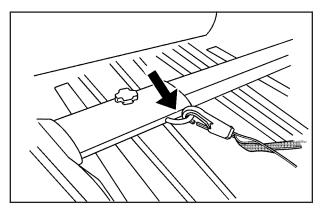
14. Clip the other end of the cargo net to the telescoping cross bar as shown.
