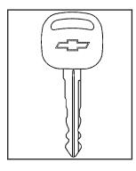
One key is used for the ignition, the doors and all locks except the center console and trailer hitch.
