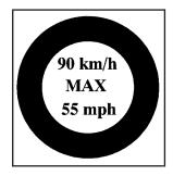
16. If the flat tire was able to inflate to the recommended inflation pressure, remove the maximum speed label from the sealant canister.
