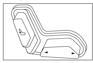
The power seat controls are located on the outboard side of the passenger's seat.
