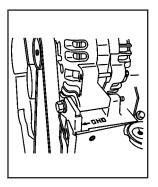
The remote negative (–) terminal is located near the power steering fluid reservoir. It is marked GND (–). See item H in the *Engine Compartment Overview on page 5-12* for more information on location.
