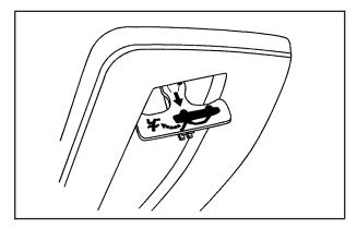
*Notice:* Using the emergency cargo cover release handle as a tie-down or anchor point when securing items in the cargo area may damage it. Use the emergency cargo cover release handle only to help you open the cargo cover.
