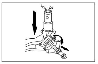
2. Be sure the unit is unlocked before pretensioning. Unlock using the key.
