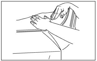
14. From the upright position, push down on the outer area of the boot cover panel where the hinges and hydraulic cylinders are located to separate it from the roof tonneau. Then, continue to push the boot cover panel down as far as it will go.
