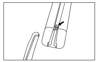
2. Locate and remove the fastener at the tailgate end of the floor track.
