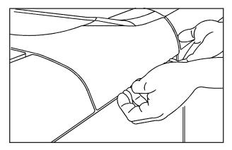
8. For steps 8 and 9, more than one person is needed to do this. One person working on each side is best. Lift up on the roof tonneau and raise it to the upright position.
