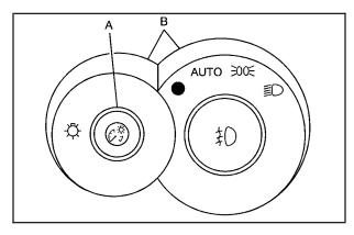
$\mathcal{G}_{\mathfrak{I}}^{\infty}$  (Interior Lamp Control): The interior lamp control (A) is located to the left of the steering wheel and is used to adjust the brightness of the instrument panel lights.
