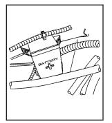
The remote positive (+) terminal is located inside a red cover in the engine compartment on the passenger's side of the vehicle. See item A in the Engine Compartment Overview on page 5-12.
