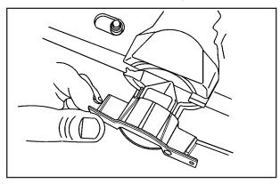
1. Remove the cover of the housing located behind the license plate area by pushing in the tabs and pulling downward.
