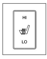
If your vehicle has this feature, the switches are located on the outboard side of the driver's and passenger's seats.
