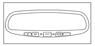
If your vehicle has this feature, the Universal Home Remote transmitter buttons are located on the automatic dimming rearview mirror. The three buttons on the left side of the mirror are the Universal Home Remote transmitter buttons.
