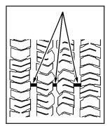
One way to tell when it is time for new tires is to check the treadwear indicators, which will appear when your tires have only 1/16 inch (1.6 mm) or less of tread remaining. Some commercial truck tires may not have treadwear indicators. You need a new tire if any of the following statements are true:
