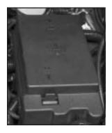
The fuse block is located under the hood in the engine compartment on the driver's side of the vehicle. See *Engine Compartment Overview on page 5-12* for more information on location.
