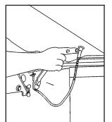
2. Disconnect the electrical connector located on the underside of the cargo cover near the front of the bed, if equipped.
