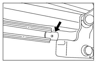
Side Rail with End Cap Removed Shown
