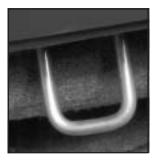
The top tether anchor is located on the back of the front passenger seat.
