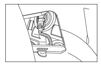
3. Turn the bulb socket counterclockwise to remove it from the headlamp assembly.
