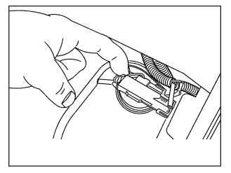
2. Remove the socket from the lamp assembly by locating and then squeezing the release tab while turning the socket counterclockwise.
