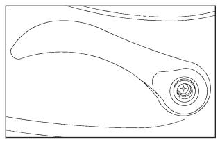
To recline the seatback, lift the lever on the outboard side of the seat cushion.
