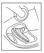
The tilt lever is located on the driver's side of the steering column, under the turn signal lever.
