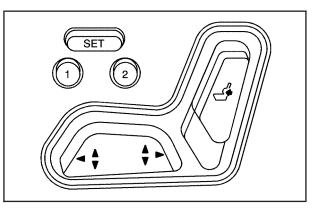
Your vehicle may have a memory driver's seat. The controls for this feature are located on the outboard side of the driver's seat and are used to program and recall memory settings for the driver's seating positions.
