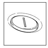
11. Remove the plastic cap located between the sun visors by turning it one quarter turn.
