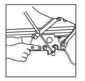
Locate and remove the bolts that hold the cargo cover in place. There is one bolt on each side near the front of the cargo area.
