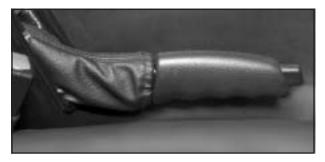
To set the parking brake, hold the brake pedal down. Pull the parking brake lever up. If the ignition is on, the brake system warning light will come on. See *Brake System Warning Light on page 3-30* for more information.
