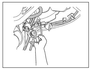
Insert the convertible top release tool and turn it to activate the emergency release. The convertible top release tool is provided by the dealer and stored in the glovebox. See your dealer if the convertible top release tool is misplaced.
