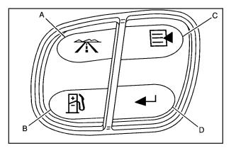
A. **7** (Trip Information): Press this button to display the odometer, trip odometer, timer, and outside air temperature.
