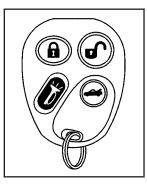
✔ (Unlock): When you press unlock, the driver's door will unlock automatically, the parking lamps may flash, the horn may sound, and the interior lights will turn on. If your vehicle has the memory seat feature and you have previously programmed a seat position, the driver's seat will move to that position when you press the unlock button. See *Memory Seat on page 2-53* for more information.
