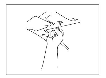
13. Insert the convertible top release tool into the latch closing mechanism between the sun visors and turn it counterclockwise until the latches are secured and the convertible top is fully closed.
