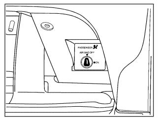
Unless the passenger's airbag has been turned off, *never* put a rear-facing child restraint in this vehicle.
