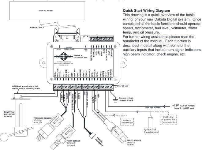
• Set up the control box to match your vehicle. The tachometer must be set to match the number of engine cylinders and the fuel gauge must be set to match your fuel sender resistance curve or the instrument system will not display correctly. The control box can read seven common fuel level sender resistance values. If your sender is not listed, the system can be programmed to a custom sender (see full manual for details).
